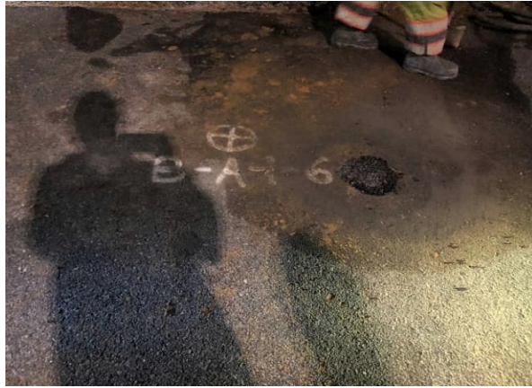
As drilled Pavement Core Location
