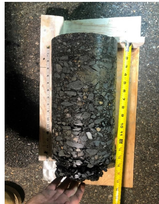
Pavement Core Sample
