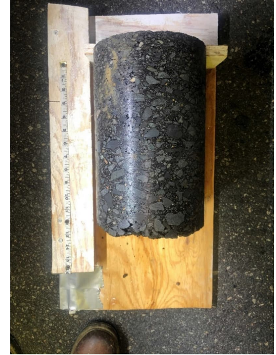
Pavement Core Sample
