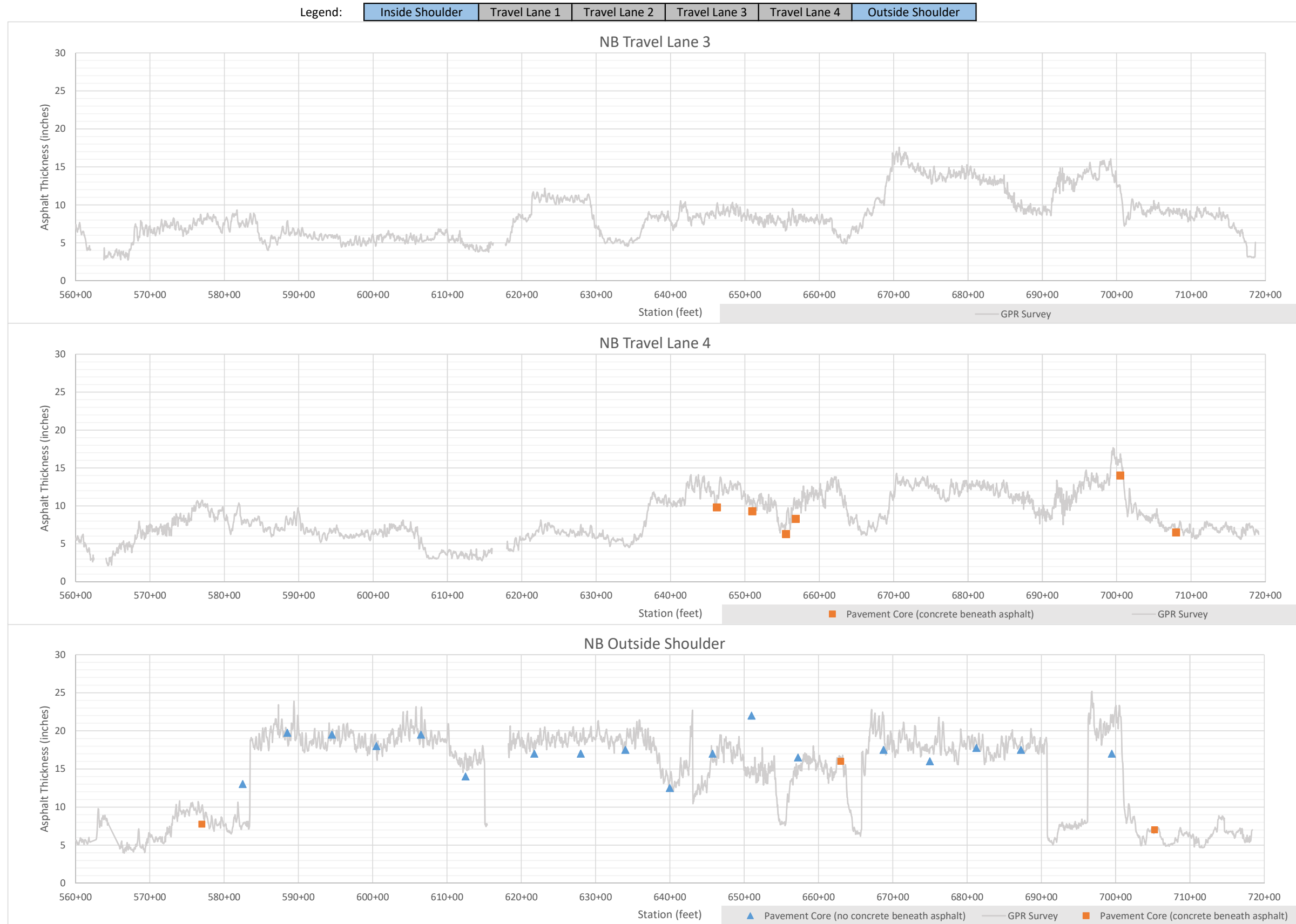
Figure C-1: 495 NB Summary of Pavement Thickness from Cores and GPR Survey
