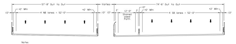
Provide 2' Min. or width necessary to meet Sight Stopping Distance on the ramps.
