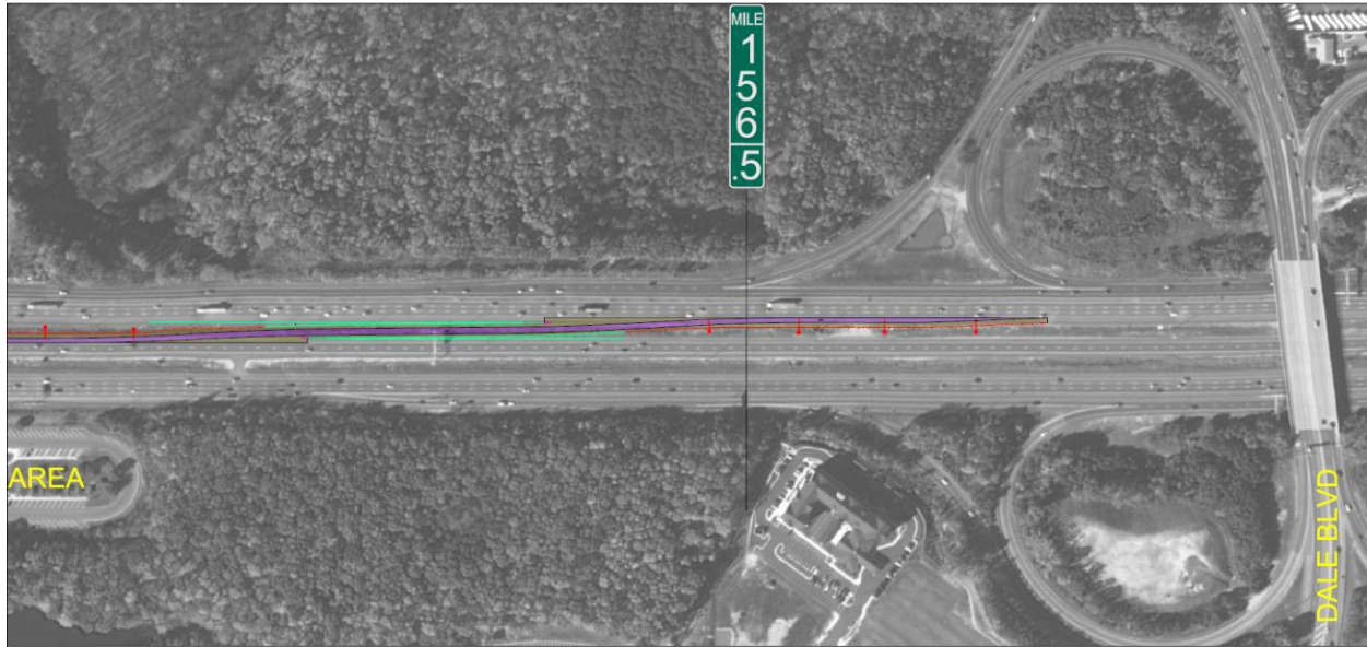
Figure 2. Project Opitz Relocated Southbound Express Slip Ramp
