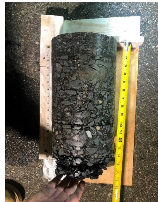
Pavement Core Sample
