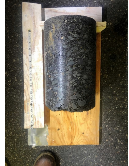
Pavement Core Sample
