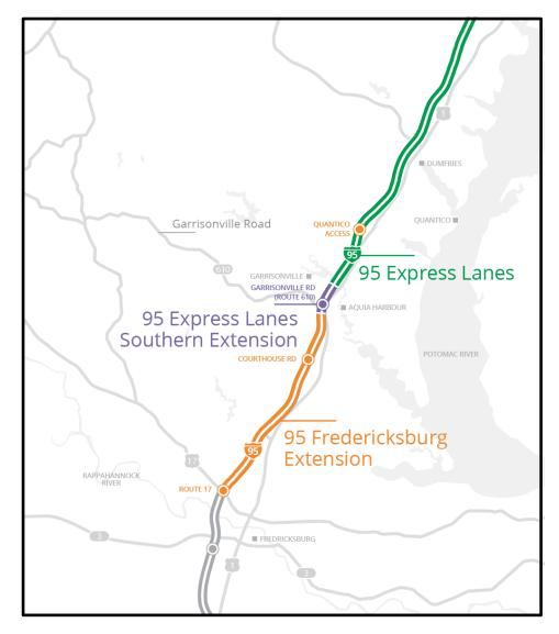
The primary objective of the Fred Ex Project is to extend the High Occupancy Toll (HOT) lanes (Express Lanes) on I-95 further south to provide additional capacity in the corridor, which will be available at no charge to HOV 3+ vehicles, and open to other permitted vehicles for a user fee (toll). The future Fred Ex Express Lanes will be subject to the same operating rules and regulations as the existing 95 Express Lanes, and when complete will operate together with the future 395
