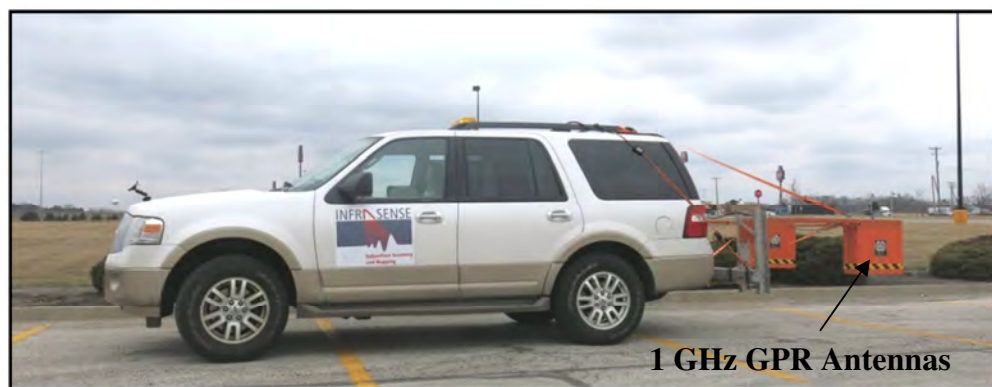
Figure 1. Field setup of GPR equipment
