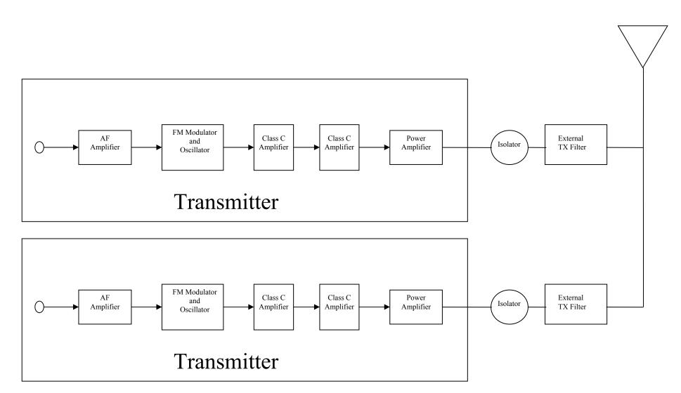
Sample Transmitter Block Diagram
